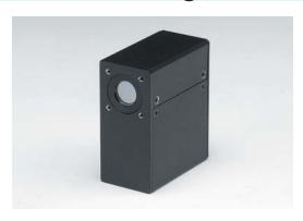
The H11890 series is a compact photon counting head consisting of a metal package photomultiplier tube along with a high speed photon counting circuit and a high-voltage power supply unit. The high voltage supply for the photomultiplier tube and the discriminator level are preset to optimum values, allowing photon counting measurement by just connecting to a PC.
