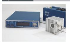
The EQ-99 Manager connects to a PC for smooth and easy control of the EQ-99X series LDLS. The front panel display allows monitoring the status of the EQ-99X LDLS including bulb operation hours. When needed, an optional shutter can be connected for advanced shutter control.
