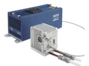
The spectral irradiance of the EQ-99X-CAL-S is calibrated and traced to national standards. Compared to traditional calibrated light sources the EQ-99X-CAL-S features a more stable spectrum and longer lifetime.
