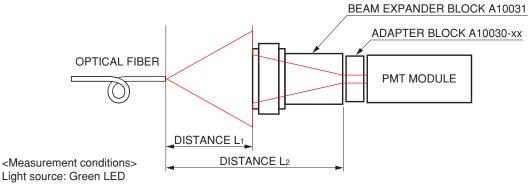
Optical fiber: NA=0.5. Core diameter=0.98 mm
