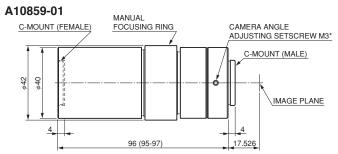
\* You can adjust the camera tilt by loosening this screw and turning the tube lens block.
