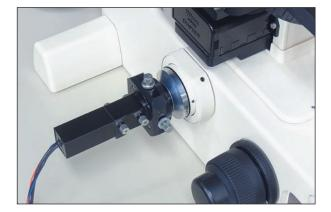
The A11027 is a holder block for mounting a pinhole. The screws can be used to adjust the pinhole's position in the XY directions. The built-in lens collimates the light that passes through the pinhole and converges the light on a photodetector.
