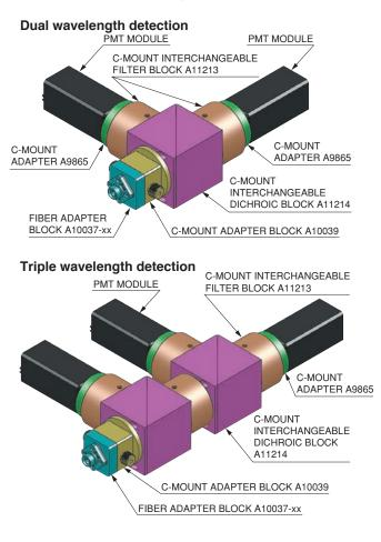
This C-mount threaded optical block is for installing a dichroic mirror for use at a 45 angle of incidence. You can use typical dichroic mirrors that are commercially available for use with microscopes.
