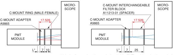
\* L is the distance from the attached end of the PMT module to the photocathode.
