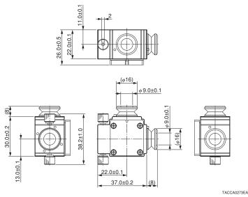
The A10035-90 is a holder block designed to hold a 15 mm cubic type beam splitter. There are M3 screw holes in the bottom of the block for holding.
