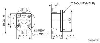
How to connect a C-mount adapter block
