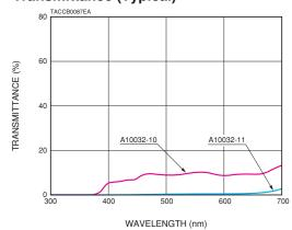
\* Transmittance characteristics are typical values and may differ depending on the production lot. A neutral density (ND) filter is included in this optical block to attenuate light levels.
