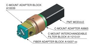
This adapter is for connecting a PMT module to a optical block or an equipment with C-mount.
