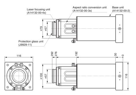
\* Tolerance is by JIS B 0405-m (Intermediate) unless specified.
