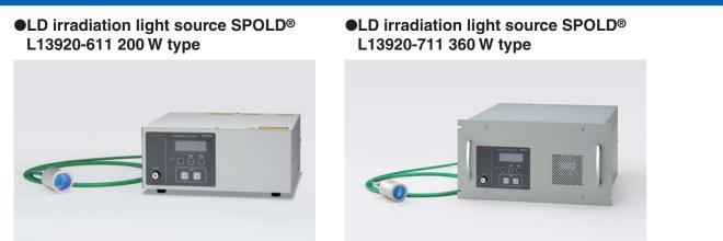
LD irradiation light source SPOLD<sup>®</sup> is a compact laser light source that combines a distilled water-cooled fiber-output laser diode module with its driver and controller circuit. It emits laser light with any desired beam diameter and profile by selecting the irradiation unit. Our product line-up also includes built-in process monitor types.
