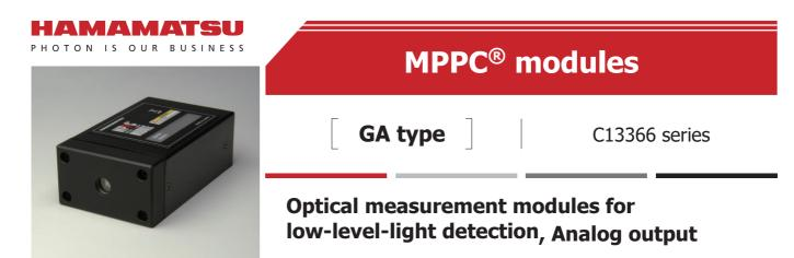
The C13366 series (GA type) are optical measurement modules capable of detecting low level light. These modules consist of a thermoelectrically cooled MPPC, a signal amplifier circuit, a high-voltage power supply circuit, and a temperature control circuit. The photosensitive area is available in two sizes of  $1.3 \times 1.3$  mm and  $3 \times 3$  mm, and the signal output is analog. Modules operate just by connecting them to an external power supply (±5 V).
