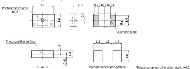
Position accuracy of photosensitive area: X, Y≤±0.2
