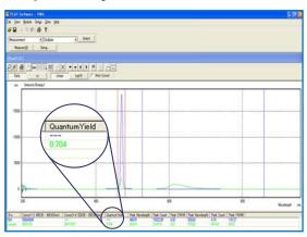
This is a basic screen for quantum yield measurements. The luminescence quantum yield is automatically calculated after measurement. Excitation and emission bands are defined by adjusting the cursors. The value of the quantum yield is displayed in the table below the spectrum next to emission intensities, peak wavelength, peak counts, and peak band (FWHM).
