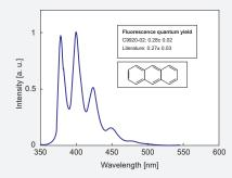
The quantum yields of fluorescence standard solutions were measured with our Absolute PL quantum yield measurement system. The fluorescence standard solutions have been used for determining PL quantum yield based on a relative method. For the most compounds, the quantum yield measured by our system shows excellent agreement with the values given in the literature, proving the high reliability of our system.
