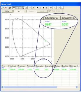
Besides displaying PL spectra and calculating quantum yields, the software also includes a function for color coordinates. In addition to the chromaticity coordinates (x, y) of the measured sample, the three stimulus values (X, Y, Z) are displayed.
