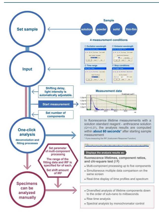
Quantaurus-Tau<sup>®</sup> includes a variety of measurement and analysis functions such as simultaneous multi-component fluorescence lifetime measurement and multi-sample data comparison.
