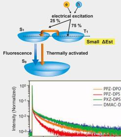
TADF (Thermally activated delayed fluorescence) is known well as the 3rd generation OLED material which is high efficiency and cost saving, furthermore can be replaced with phosphorescence material. The data shows the example of fluorescence lifetime measurement of blue TADF material. In order to achieve the high efficiency, the molecule design is the important factor to minimize the energy gap of excited singlet state (S<sub>1</sub>) and excited triplet state (T<sub>1</sub>).
