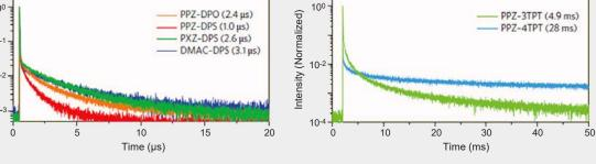
Delayed fluorescence of TADF material results in that small gap of  $\Delta$ Est, which is defined as the energy gap of S<sub>1</sub> state and T<sub>1</sub> state, is in the microsecond range. On the other hand, wide gap of  $\Delta$ Est is in millisecond range.
