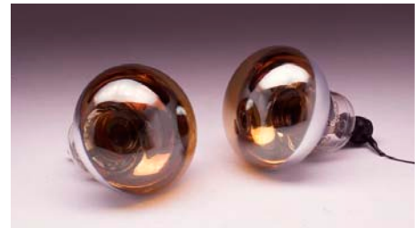
Large diameter 20-inch PMTs
