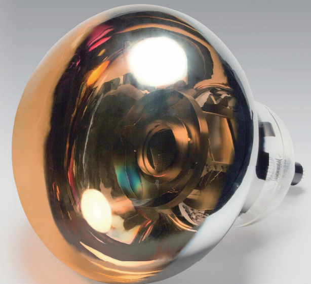
▲ New 20-inch-diameter PMTs
