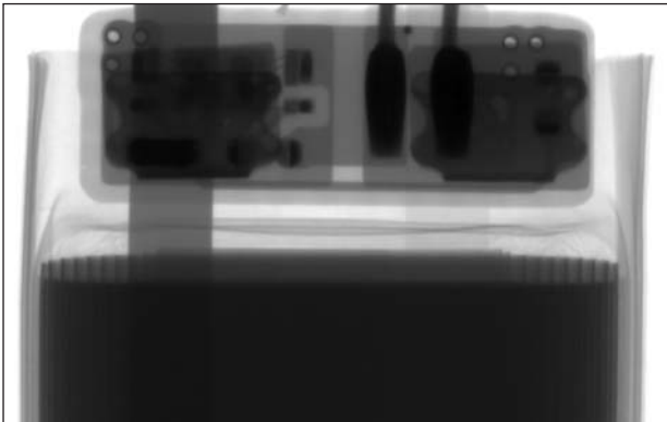
Lithium-ion battery and protection circuit
