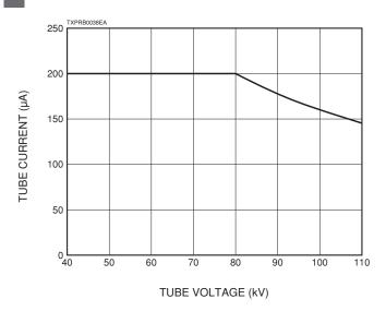
\* The X-ray tube voltage guaranteed range is 40 kV to 110 kV.
