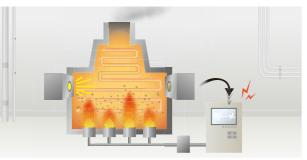
Flue gas monitor Analysis of SOx and NOx in gases emitted from factories and the like.
