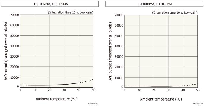
A/D output is the sum of the sensor and circuit offset outputs and the sensor dark output.
