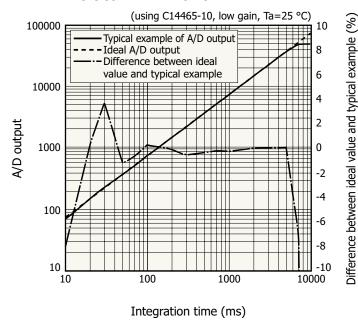
A/D output is the output with dark output is subtracted when light is input. The difference between the ideal value and typical example contains a measurement error. The smaller the A/D output, the larger the measurement error.
