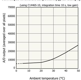
$\mbox{\ensuremath{A/D}}$  output is the sum of the sensor and circuit offset outputs and the sensor dark output.
