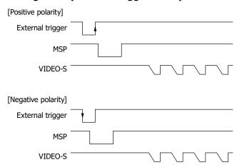
Delay time from when an external trigger is input to when exposure is started=30 ns
