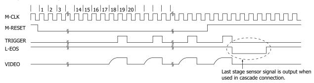
Timing chart of second and subsequent stage sensors when used in cascade connection
