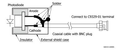
Anode: Connect to the shield wire of the cable and shield case.
