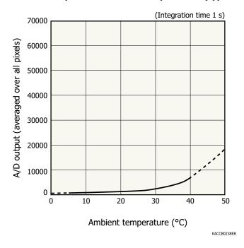
A/D output is the sum of the sensor and circuit offset outputs and the sensor dark output.
