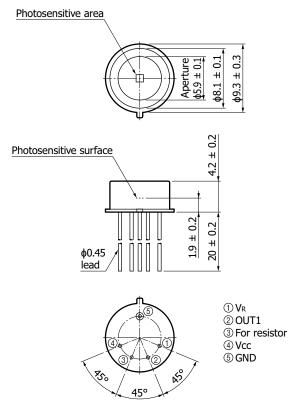
Note: Please connect the same resistance to the terminal 23. Make sure to connect a bypass capacitor (0.1 to 10  $\mu$ F) to the supply voltage 4 to prevent oscillation.
