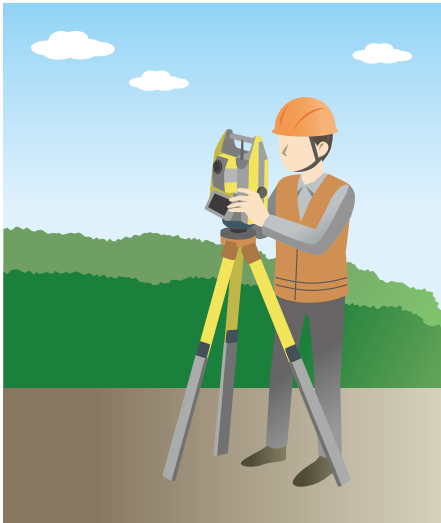
The measurement object is irradiated with laser light, and the reflected light is detected by a photosensor with front-end IC to measure distance.
