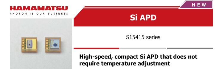
The S15415 series is a gain-stabilized APD (GS APD) with a built-in temperature compensation function inside the sensor. This realizes constant gain without the need for temperature adjustment. It is suitable for laser monitors of optical rangefinders used in a wide range of applications, from consumer to industrial.
