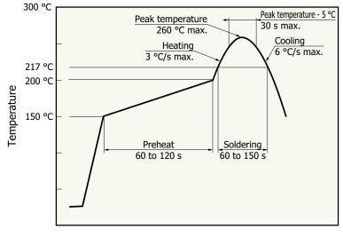
• After unpacking, store in an environment at a temperature of 30 °C or less and a humidity of 60% or less, and perform reflow soldering within 4 weeks.
