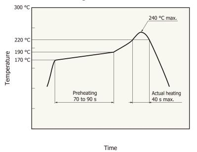
• This product supports lead-free soldering. After unpacking, store it in an environment at a temperature of 30 °C or less and a humidity of 60% or less, and perform soldering within 24 hours.
