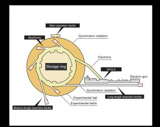
Internal structure of SPring-8
