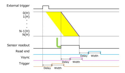
Figure 11-23 Programmable timing output (Top to bottom readout)
