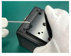
3. Confirm the base plate is firmly fixed.
