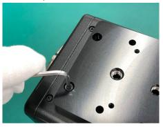
Fasten screws by hexagonal wrench while holding the camera.
