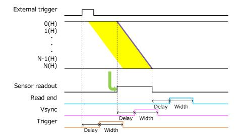
Figure 11-12 Programmable timing output
